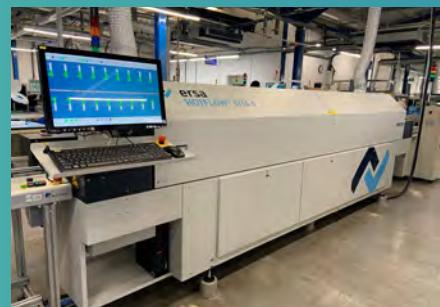
We have taken delivery of a second new reflow oven, widely regarded as the best in its class, with the 7 zone heat tunnel and a process length of over 4 metres. It offers the highest throughput, optimised energy balance, best process control and maximum machine up-times, with the "e" standing for efficiency.
